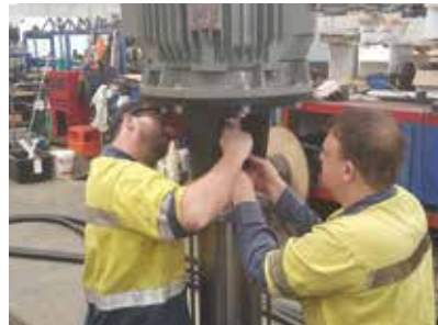
Custom build of water transfer pump package
