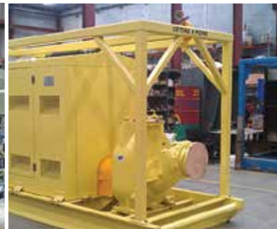
Design and build of diesel driven water transfer pump package
