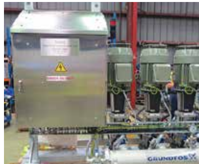
Design and build of 3-unit wash down pump package
