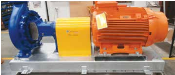
Design and manufacture of 150kW ISO pump set
