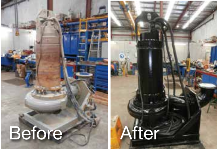
Overhaul and upgrade of 140kW Grundfos S2 pump
