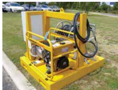
Custom build of bore water sampling package
