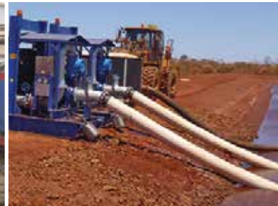
Design and build of 16 diesel driven water transfer pump packages
