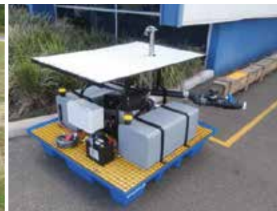
Custom build of self-priming, diesel-powered pump package
