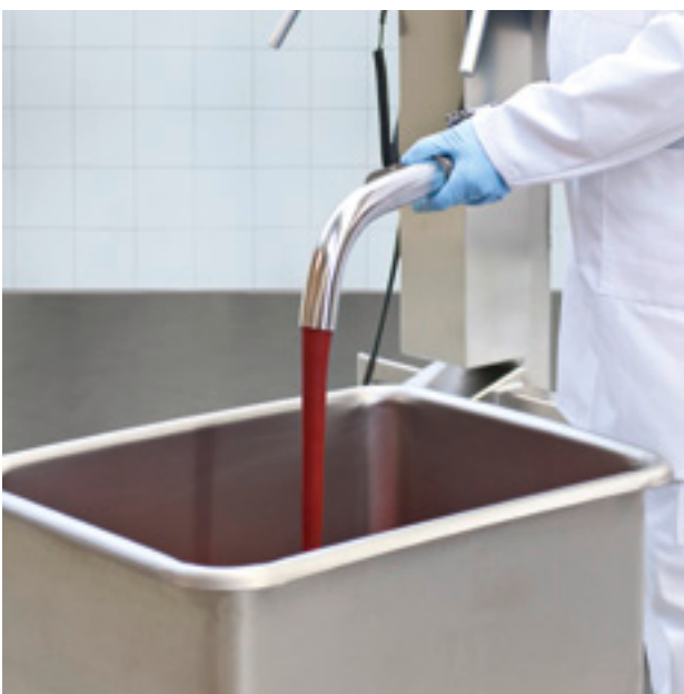
Basic food such as vegetable and fruit concentrates can be gently transferred with low-shear.
