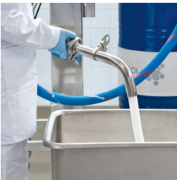
Gentle, continuous pumping based on the example of Vaseline.
