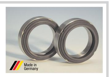
The medium lubricated mechanical seals type KPS3 and KPG3 are specially designed for the application in Sunflo Pumps type P-3000. Identical dimensions with the original seals allow easy installation and interchangeability.
